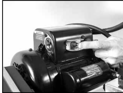
(B) Move the Voltage Change Switch to the desired voltage setting.
