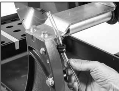
(A) Insert cooling transfer hose through loop.
