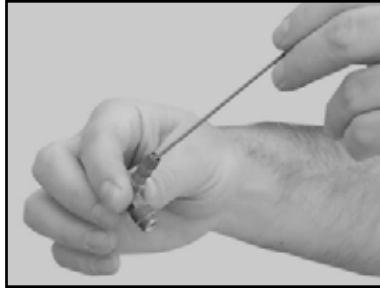
(E) Clean the Blade Guard Intake Fitting
