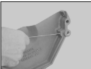
(G) Rod Cooling Channels and recheck flow
