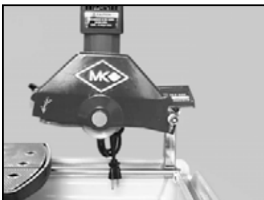
(A) Loosen the Blade Guard Retaining Wingnut
