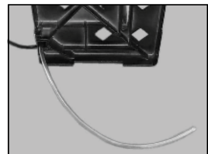
(C) Remove the Cooling Transfer Tube from the Blade Guard inlet. Inspect for blockage.
