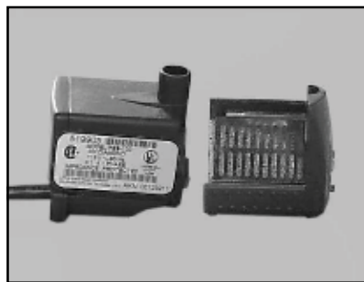
(B) Remove the pump suction screen and clean the Water Pump of all debris.
