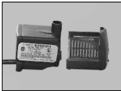
(D) Remove the pump Suction Screen and clean the Water Pump of all debris
