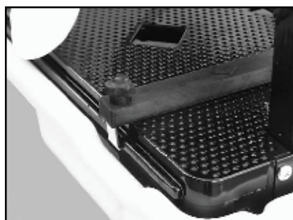
(D) Verify the Rear Guide is properly seated under the rear guide Slot
