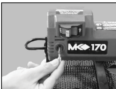
(E) Align and install the new Motor Brush.
