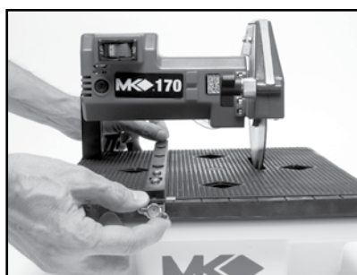
(B) Place the adjustable Cutting Guide onto the Cutting Table with the Front Guide into the front Guide Slot and the Rear Guide in the rear Guide Slot
