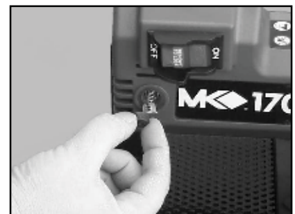
(F) Install Motor Brush Cap and tighten using a Flat Head Screwdriver.
