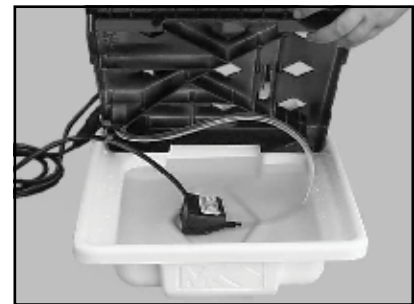
(I) Remove the Cutting Table for the Water Pan
