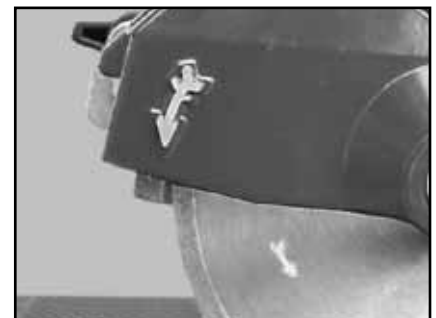
(F) Verify the Directional Arrow of the Blade faces outward and matches the Directional Arrow of the Blade Guard
