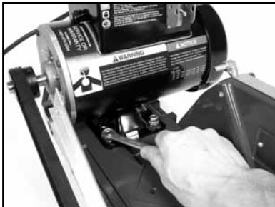
(P) Tighten the four motor mounting bolts.
