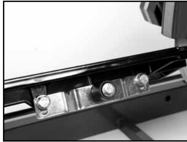
(B) Lubricate the Roller Wheel Assembly.
