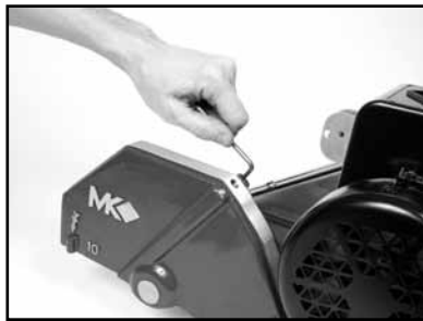
(G) Remove the Cooling Channel cover screws.
