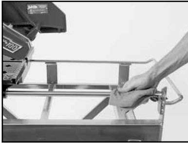
(A) Lubricate the Guide Bar.
