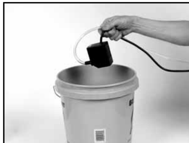
(B) Place the Water Pump in an external container and fill until water completely covers the Water Pump suction.
