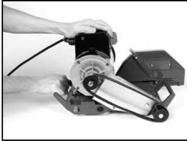
(J) Push the motor toward the front of the Cutting Head to loosen the V-Belt.
