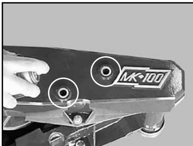
(J) Lubricate the Cutting Head Adjustment Knob retaining holes.
