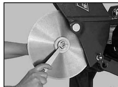
(F) Depress and hold the Shaft Lock button and tighten Retaining Nut.
