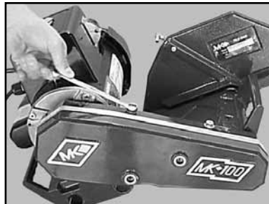
(Q) Install the Belt Guard.
