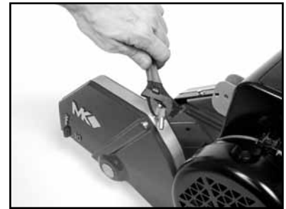
(F) Remove the Blade Guard Intake Fitting and check.
