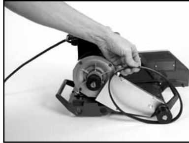
(K) Remove the V-Belt.
