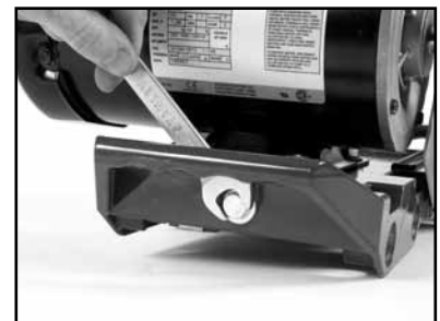
(I) Loosen the Motor Adjustment Strap.
