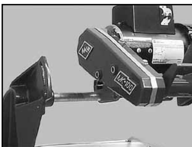
(G) Install the Cutting Head in rear Pivot Hole (Cutting Head Adjustment pg 25).
