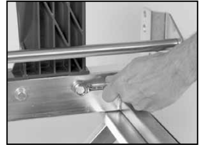
(C) Loosen the Retaining Bolts.
