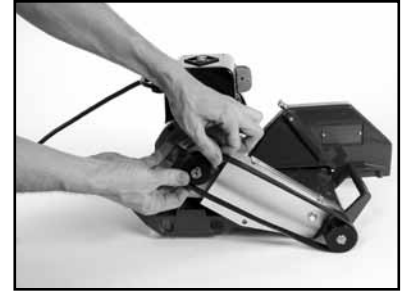
(L) Install the new V-Belt (MK Diamond Part No. 158194).
