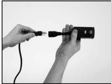
(B) Plug MK-100 into GFCI.
