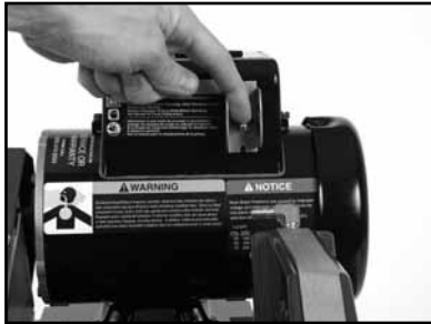
(A) Ensure the ON/OFF Switch is in the OFF position.
