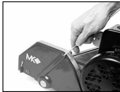
(H) Rod Cooling Channels and recheck flow.
