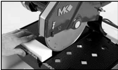
(A) Cut the Dressing Stick 7 or 8 times to dress the Blade.
