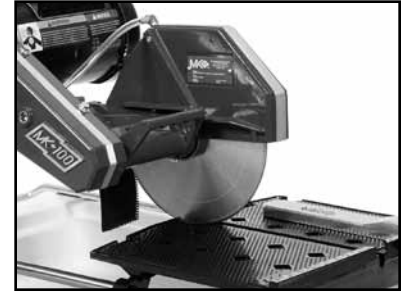
(F) Install Diamond Blade. Set cutting depth approx. 1/4 to 1/2 inch below the surface of the Movable Cutting Table.
