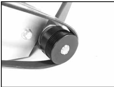
(M) Verify the V-Belt is seated in the grooves of both pulleys.
