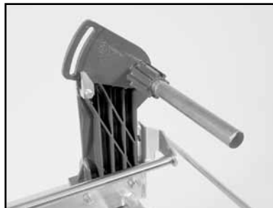
(K) Lubricate the Cutting Head Pivot Shaft.
