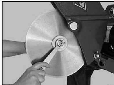
(B) Remove Retaining Nut and Outer Flange, depress and hold the Shaft Lock hold button and loosen.
