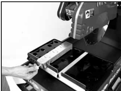
(A) Set the adjustable Cutting Guide.
