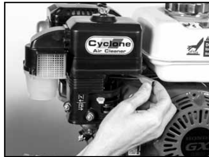
(B) Move the Throttle Level to lower blade speed. Refer to your specific Engine Manual.
