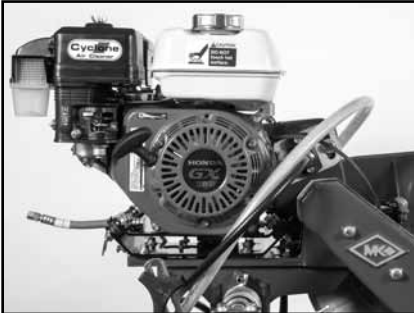
(A) Level Cutting Head and motor.
