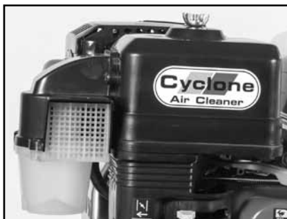
(H) Check Air Filter for cleanliness. (See Engine Manual)
