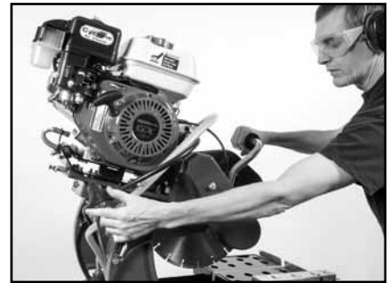
(I) Unlock Cutting Head.
