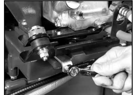
(C) Verify engine adjustment Straps are tight.
