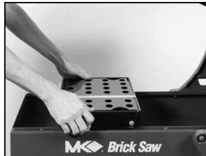
(B) Seat movable Cutting Table roller wheels on saw Guide Rails
