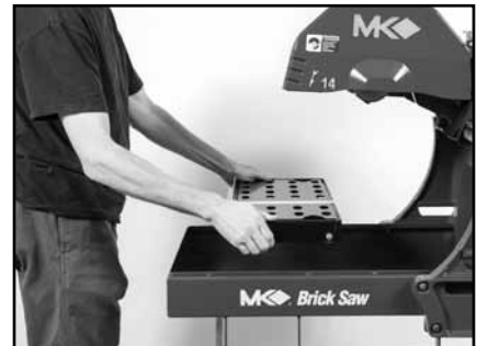
(F) Install the movable Cutting Table.
