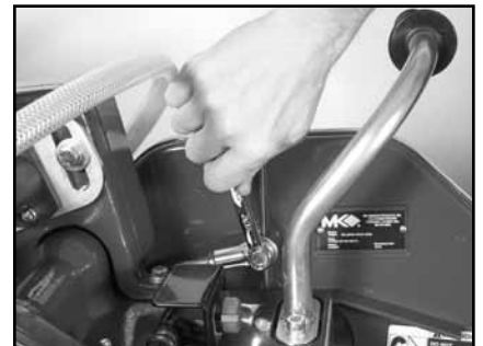
(X) Install the Blade Guard Adjustment Bar.
