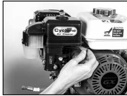
(H) Move the Throttle Lever to lower blade speed.
