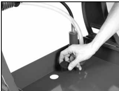
(A) Install the Drain Plug and fill Water Basin.
