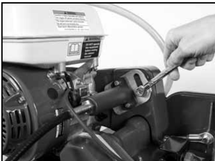
(V) Locate Water Pump Pivot Plate loosen retaining bolts.
