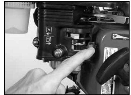
(C) Place Fuel Valve in the OFF position.
