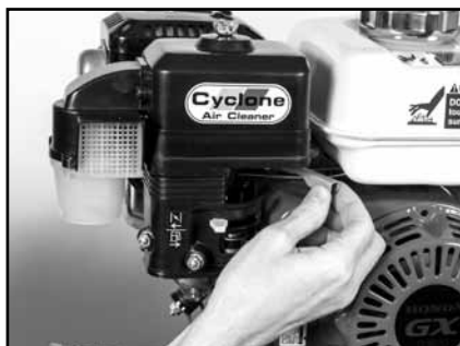
(A) Move the Throttle Lever to lower blade speed.
