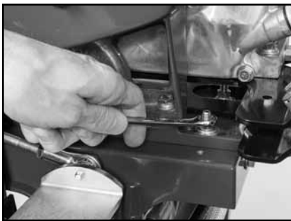
(D) Loosen engine mounting plate. If re-tensioning, go to Step J. 5 bolts, 4 under motor, 1 to left of power switch.
