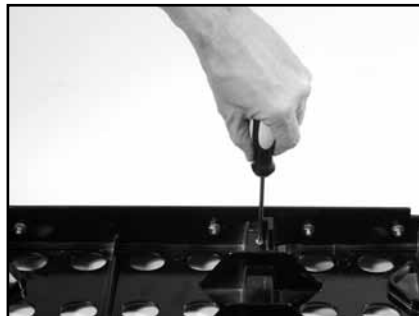
(E) Tighten screw to secure new Wooden Strip.
