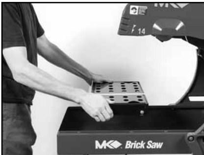
(A) While holding the front, position movable Cutting Table roller wheels above Guide Rails
