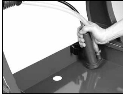
(B) Remove Water Pump from clamp.
