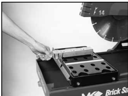
(A) Set the adjustable Cutting Guide.
