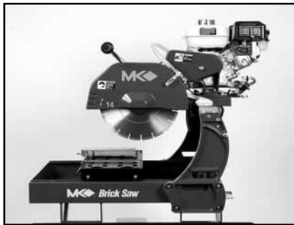
(E) Inspect MK-2000 Gas Saw for general damage, loose connec- tions and hardware.
