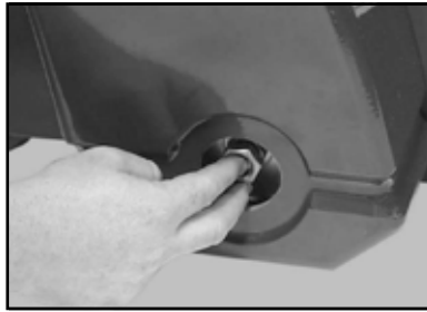
(K) Install the Shaft, Inner Retaining Nut.
