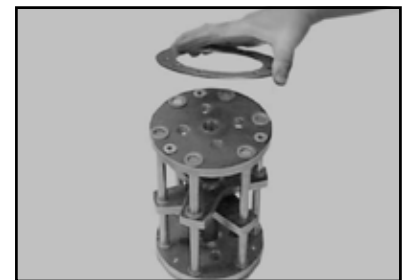
(C) Remove the Drum Retaining Ring.
