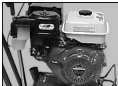
(E) Check Fuel Line (2-Year Maintenance Only, Shop Maintenance Required).
