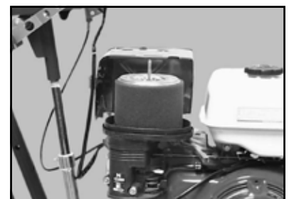
(F) Clean engine Air Filter (See Engine Air Filter Inspection Cleaning and Replacement).
