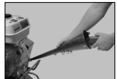
(F) Fill the Oil Reservoir (See Engine Manual).
