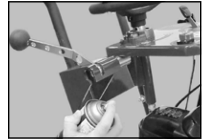
(I) Lubricate the Engage/ Disengage Pivot Shaft.
