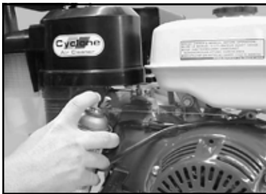
(K) Lubricate engine Throttle Linkage.
