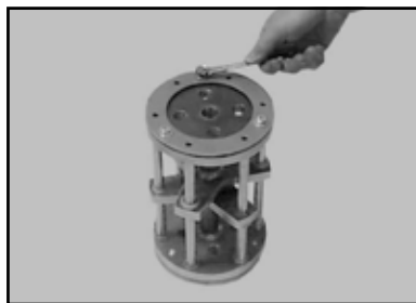
(B) Remove the 3 Retaining Screws using a 7/16-inch wrench.
