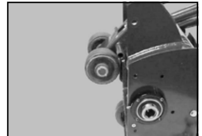
(F) Remove the Rear Wheel Retaining Cotter Pin, Shim Washer and Rear Wheel from each side of the Assembly.
