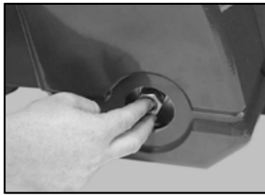
(N) Install the Shaft, Outer Retaining Nut.
