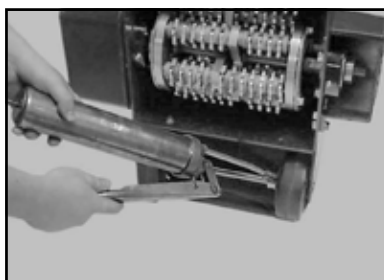
(E) Lubricate the Front Wheel Assembly Bearings.
