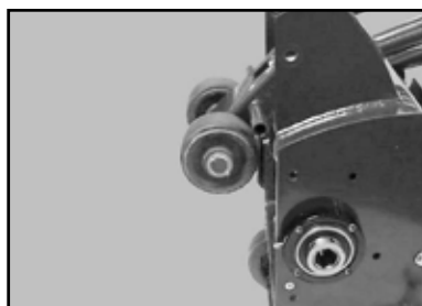
(H) Install the new Rear Wheel, Shim Washer and Cotter Pin on each side of the Assem- bly.
