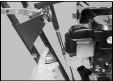
(J) Lubricate and clean the Depth Control Screw.
