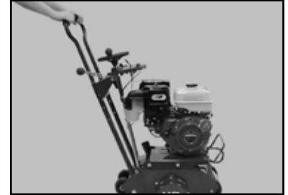
(C) Raise or lower the Handlebar as needed.
