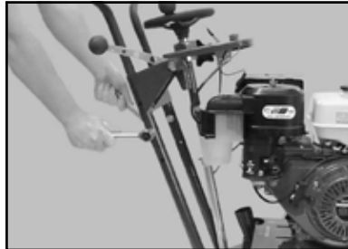
(E) Install the Retaining Bolts and tighten using 9/16 wrenches and/or sockets.
