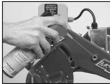
(K) Lubricate the Cutting Head Adjustment Knob retaining holes.
