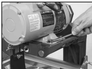
(P) Tighten the motor mounting bolts.
