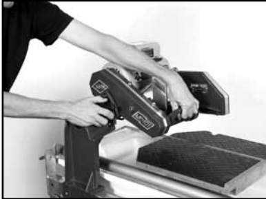
(A) Loosen Cutting Head Adjusting Knob.
