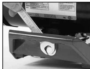
(H) Loosen the Motor Adjustment Strap.
