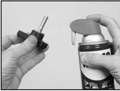
(J) Lubricate the Cutting Head Adjustment Knob.
