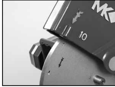
(B) Check for proper blade rotation.
