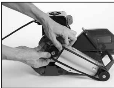
(K) Install the new belt.
