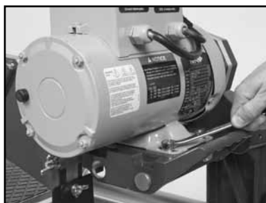
(G) Loosen the motor mounting bolts, if re-tensioning only go to step M.
