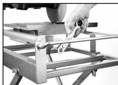
(B) Tighten Guide Bar Retaining Bolts.
