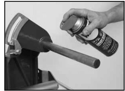
(L) Lubricate the Cutting Head Pivot Shaft.
