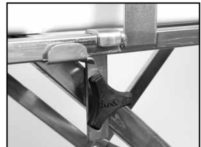
(C) Ensure saw frame is positioned correctly
