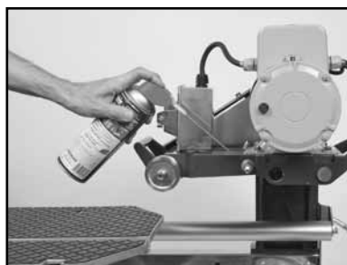
(H) Lubricate the Blade Guard Pivot Shaft.
