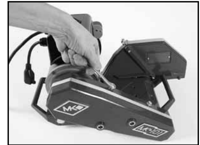
(C) To remove the Belt Guard, loosen the two top bolts on the belt guard.
