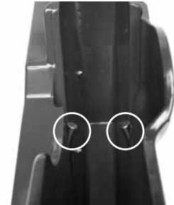
(C) Run the MK-101 until clear water is seen at the blade cooling ports (Approx. 1 min- ute).
