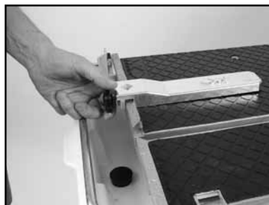
(B) Set the Adjustable Cutting Guide to cut a 1/16-strip.
