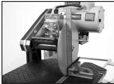
(B) Position Square on Movable Cutting Table against the Diamond Blade.
