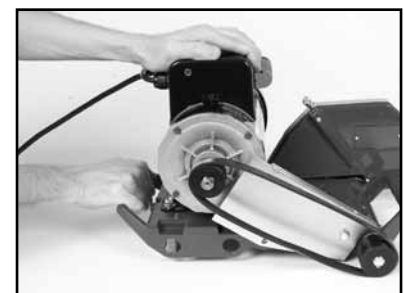
(I) Push the motor toward the front of the Cutting Head to loosen the belt.
