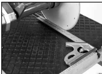
(A) Move the Cutting Table back and forth to verify Blade is even across all points of Square.
