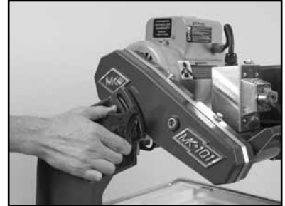
(C) Tighten the Adjusting Knob.
