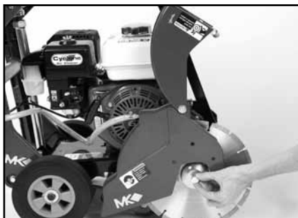
(G) Install the Blade Retaining Bolt.
