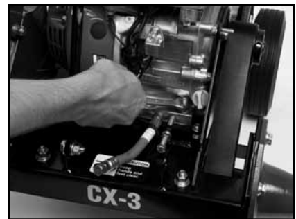
(O) Tighten the Engine Mounting Bolts.
