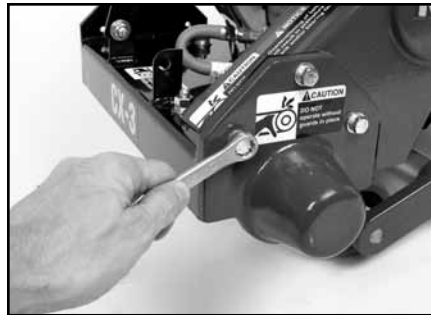
(K) Install the Blade Shaft Cover.
