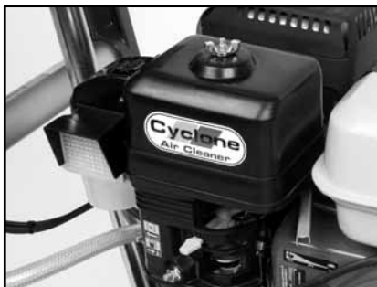
(A) Clean the Air Filter. Refer to Engine Manual for details.
