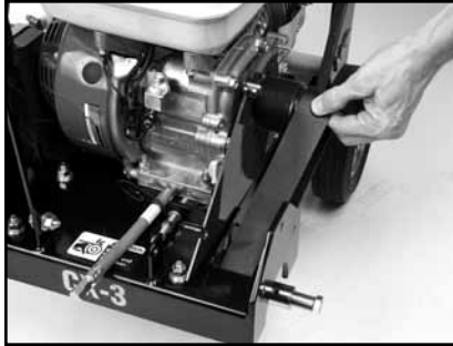
(H) Remove the old belt from the Engine and Blade Shaft Pulleys.
