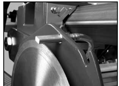
(C) Run the saw until clear water is seen at the blade cooling ports (Approx. 1 minute).
