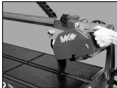
(E) Raise Cutting Head. Retighten Cutting Head Height Lock.
