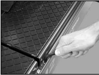
(D) Remove all Retaining Screws using the Allen Wrench provided.
