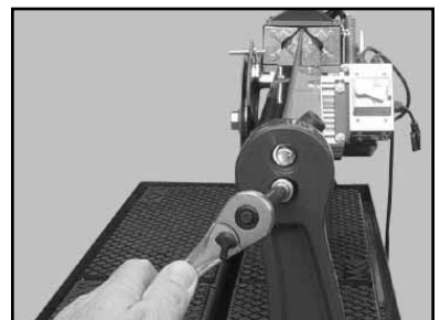
(F) Loosen the four Guide Rail Adjusting Screws using a 1/2-inch socket.
