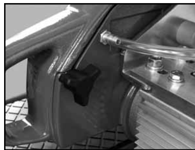
(E) Loosen the Blade Guard Retaining Knob.
