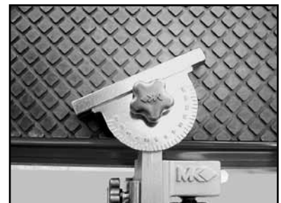
(C) Set the desired Cutting Angle and tighten the Retaining Knob.
