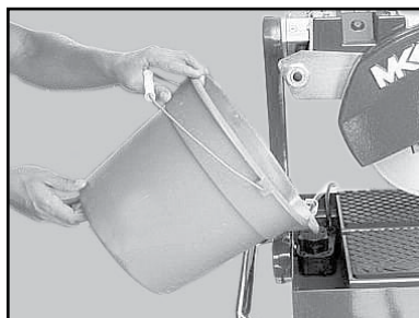
(B) Fill the Water Basin until water completely covers the Water Pump suction.
