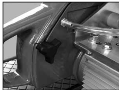
(Q) Tighten the Blade Guard Retaining Knob.
