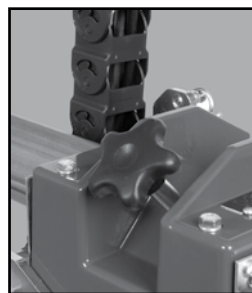
(H) Tighten the Cutting Head Locking Knob.
