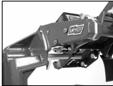
(B) Remove the Cutting Head (See Adjusting the Cutting Head).
