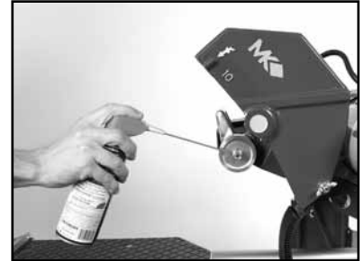
(C) Lubricate the Arbor Shaft.
