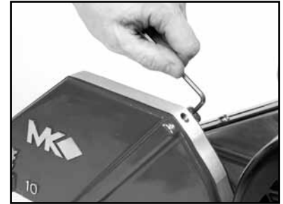
(F) Remove the Cooling Channel cover screws. Go to step G.
