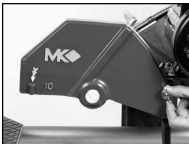
(G) Remove the Blade Guard.
