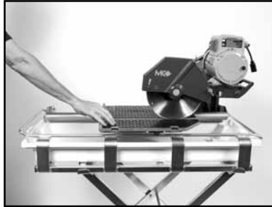
(B) Verify the Movable Cutting Table moves freely.
