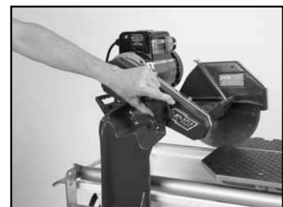
(C) Tighten the Adjusting Knob.
