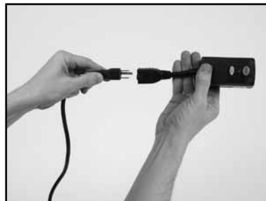
(B) Plug MK-100 into the GFCI.
