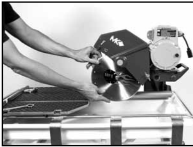
(A) Remove the Diamond Blade
