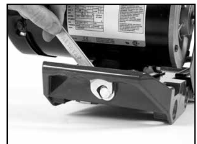
(I) Loosen the Motor Adjustment Strap
