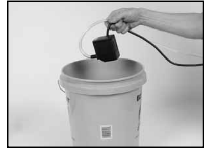
(C) Place Pump into a bucket of water and check flow. If flow exists, go to Step D.
