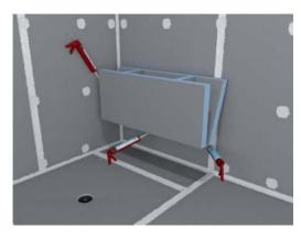
wedi Joint Sealant has to be applied on all bench carrier surfaces with contact to the walls or floor. Apply weight to the bench carrier when placing it into positon so that the wedi Joint Sealant may form a tight adhesion and seal while kept under pressure for a minimum of 30 minutes. The joint sealant should be applied in continuous beads and  $\frac{1}{2}$  thick. All excess sealant should be wiped flat right away using a putty knife.
