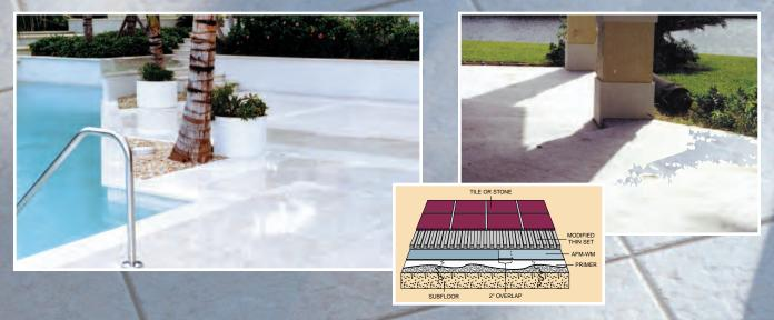
AFM-WM Waterproofing Membrane incorporates a 2" overlap guide on one side of the sheet for waterproofing. The 2" flood coated lap allows an adhesive-to-adhesive cohesive bond between subsequent sheets of membrane. Once the cohesive bond occurs, AFM-WM turns into a monolithic or single-ply membrane across the entire surface being waterproofed.
