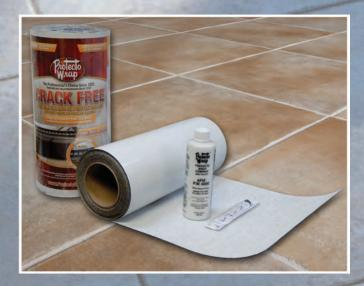
For Crack Isolation, we recommend using a membrane that will cover the crack a minimum of 1-1/2 times the width of the tile being used and a width sufficient to allow any tile spanning a crack to rest completely on the membrane. AFM is conveniently packaged in a 25 square foot kit, a 75 square foot kit or a 125 square foot kit, which include our water based primer for indoor use.
