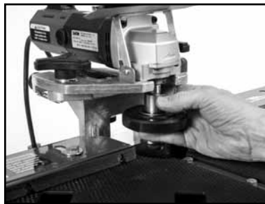
(B) Place the tool on the motor spindle and spin it on by hand.
