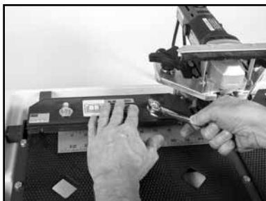
(G) Holding the straight edge firmly in place, slide the left fence into contact with the straight edge and tighten the two bolts that hold it.
