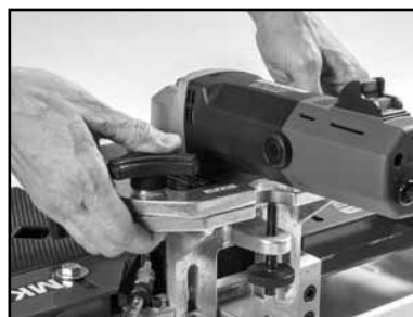
(B) Place the cutting head in position and replace the bolts and washers, through the vertical slots in the cutting head slide.
