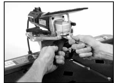
(C) Then using the two wrenches provided, tighten it up. The smaller wrench fits the flats on the motor spindle to hold it from turning, while the larger 1" wrench fits the profiling tools.
