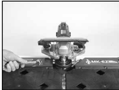
(E) Loosen the two bolts on both fences and slide them towards the back of the machine.
