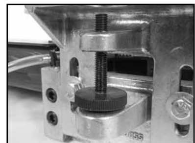
(C) Slide the head down, until the end of the vertical adjustment screw is sitting in the hole in the cutting head mount.
