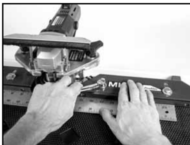
(H) Now holding the straight edge in contact with the left fence (and guide bearing), bring the right fence up to touch the straight edge and tighten it in place.
