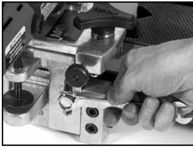
(D) Tighten the screws using a 9/16" wrench (not included).
