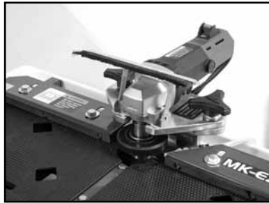
(A) Flip the splash guard brush up out of the way.
