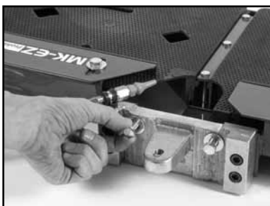
(A) Remove the two bolts and washers at the back of the cutting head mount.
