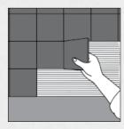
Keep tiles and joints straight and uniform. Use tile spacers if desired.
