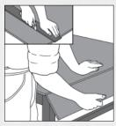
Power saw: Use a low-RPM portable saw with 3-1/2" carbide-tipped blade. To make cutouts for pipes and fixtures, use utility knife to cut through mesh on both sides of panel and punch out with a hammer from back side. Or, use an electric drill with a hole-saw bit.
