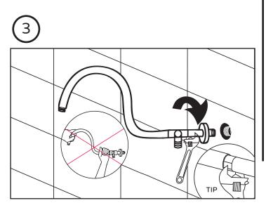
Insert threaded pipe into female wall fitting and tighten securely. TIP: Use diverter body to tighten by hand or use a pipe wrench on inlet piece closest to wall.
