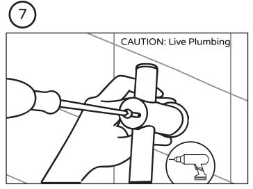
Mark wall for two mounting holes. Before drilling ensure no live plumbing can be damaged. Slowly drill 1/4" (6mm) wide by 1" (25mm) deep holes 22  $^{\rm 5/8}$  inches (575mm) apart.
