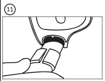
Align tab on soap dish with slot on sleeve and push soap dish down until flush. Slide lower mount (7) over slide bar and secure set screw (8).
