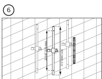
Hold adjustable slide bar (6) in desired mounting location. Evaluate range of adjustment and potential interference of handshower hose (15). Use level to assure shower pipe is straight.
