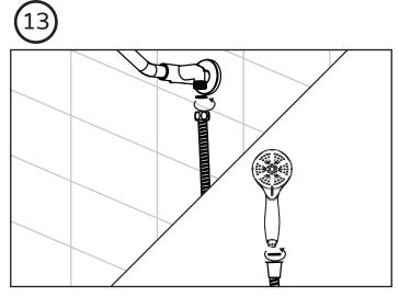
Place washer (2) in hex end of hose (15) and connect to diverter outlet. Place washer (2) in tapered end of hose and connect handshower (13). Place handshower onto holder.
