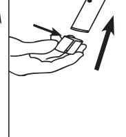
Slide ABS soap dish (12) onto slide bar followed by narrow end of tapered nylon sleeve (11).
