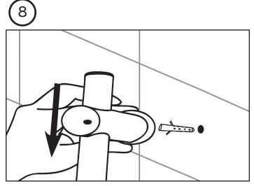
Insert wall anchors (10) until flush with wall. Slide top mount (7) over slide bar.
