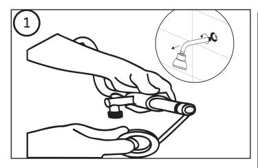
Remove existing shower arm and shower head. Wrap threads of shower pipe with Teflon tape and/or pipe sealant to make ensure no leaks.
