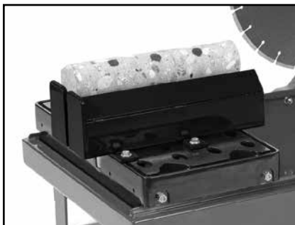
(A) Install Core Holder on to table. (MK-2002E Saw)
