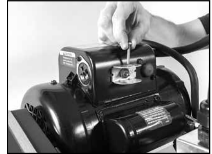
(B) Reinstall the locking bolt and replace the nut.
