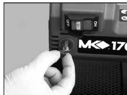
(C) Remove Motor Brush Housing Cover.
