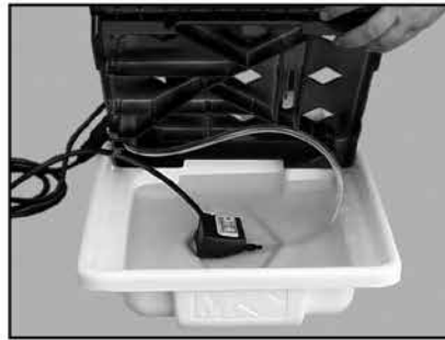
(E) Place the Water Pump in the Water Pan-ensure the pump suction is covered.
