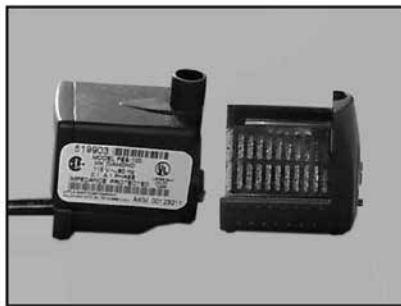
(D) Remove the pump Suction Screen and clean the Water Pump of all debris.
