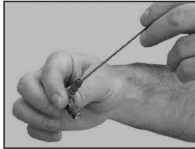
(E) Clean the Blade Guard Intake Fitting.
