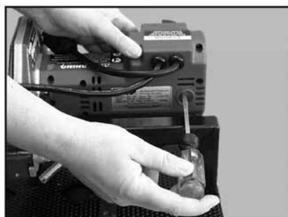
(G) Install the Second Motor Brush (Repeat Steps B to F).
