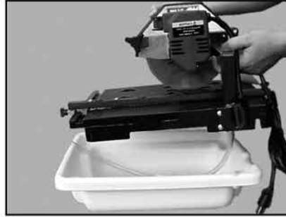
(B) Remove the Cutting Table from the Water Pan.
