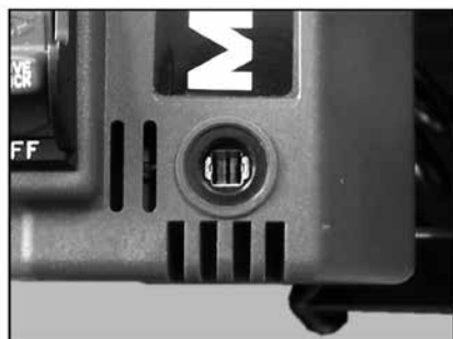
(D) Clean the Motor Brush Housing using a Q-tip.
