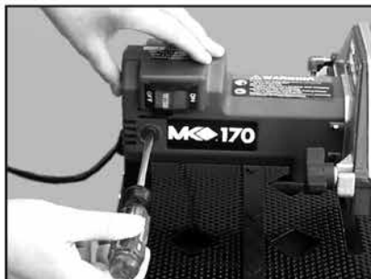
(B) Locate and Remove One Motor Brush Cap using a Flat Head Screwdriver.
