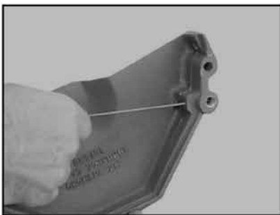
(G) Rod Cooling channels and recheck flow.
