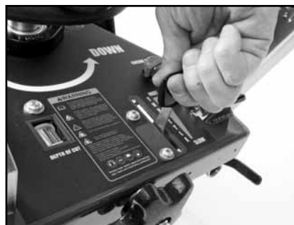
(G) With the engine running adjust the throttle approximately half-way.
