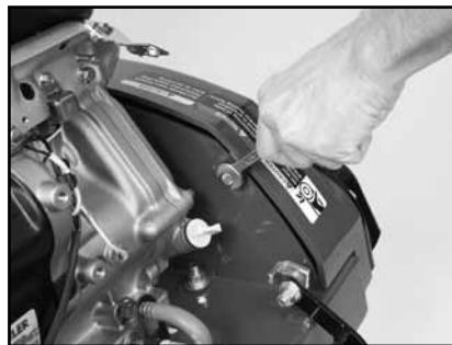
(Q) Install the Belt Guard and Belt Guard Retaining Bolts.
