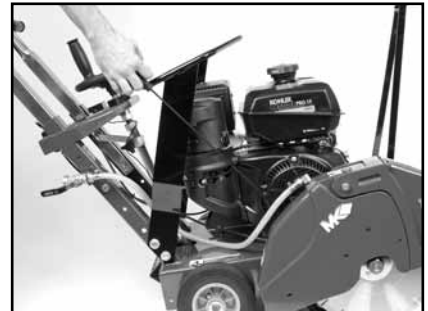
(F) Start the Saw using the Engine Start procedure in the engine manual.
