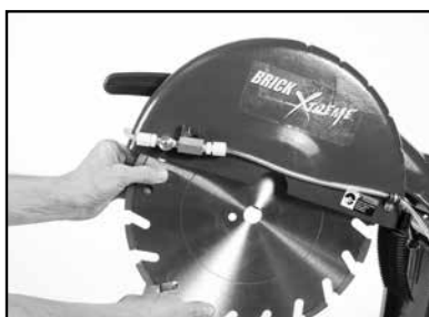
(B) Remove blade from Motor Shaft.
