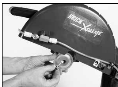
(B) Remove retaining screw and Outer Flange.
