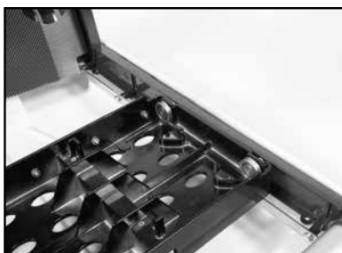
(E) Clean the Movable Cutting Table Roller Wheels and Guide Rails.
