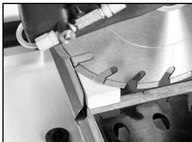
(B) Set adjustable Cutting Guide to cut 1/16-inch strips. Position Dressing Stick and cut until blade is dressed. Turn OFF saw.
