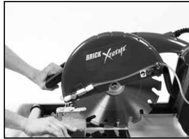
(B) Position work below Cutting Head.
