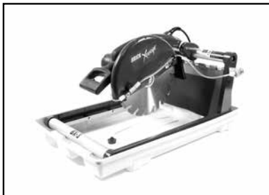
(A) Place saw in Water Pan (if applicable).
