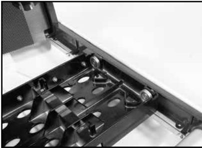
(A) Check Guide Rails clean.
