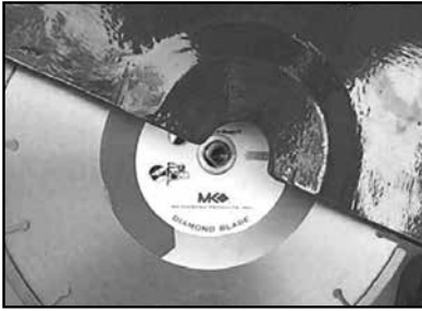
(D) Verify blade is correct for material being cut.
