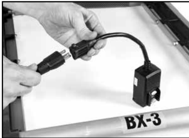
(A) Plug GFCI into BX-3.
