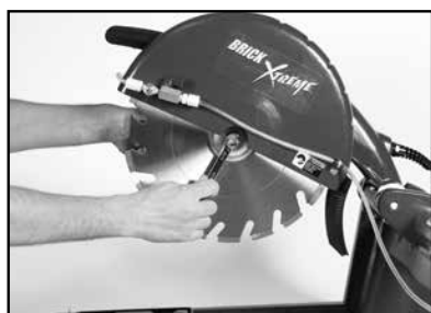
(A) Remove retaining screw and Outer Flange.
