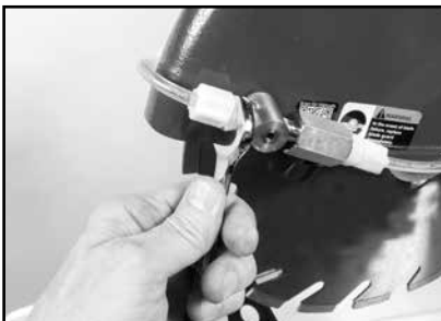
(A) Loosen tube fitting.
