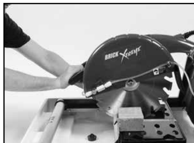
(B) Lower Cutting Head to begin cutting.
