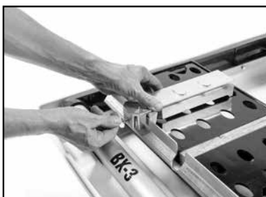
(A) Set edge of Cutting Guide to desire cut length on Ruler/ Stop.
