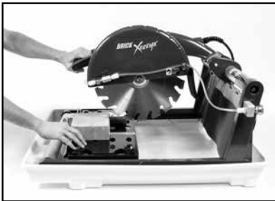
(A) Depress Trigger Switch to start cut.
