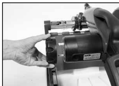
(D) Reinstall Filter into Filter Cap and onto motor.
