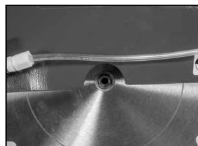
(C) Install blade under Blade Guard and onto Motor Shaft.
