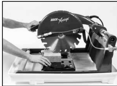
(B) Lower Cutting Head 1/4 - 1/2 inch during push stroke.
