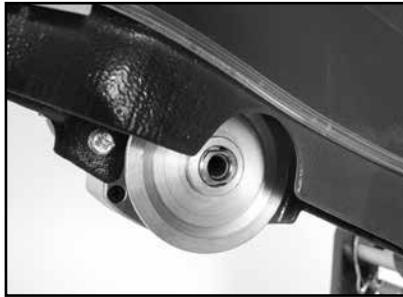
(B) Check for Roller Wheel damage.
