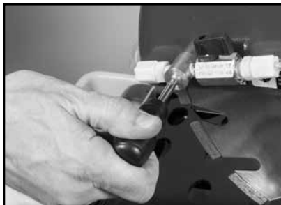
(B) Remove screw fitting.
