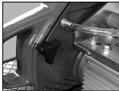
(Q) Tighten the Blade Guard Retaining Knob.
