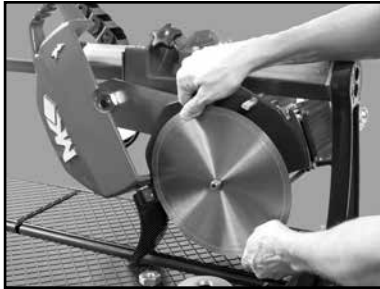
(K) Install Diamond Blade onto Blade Shaft
