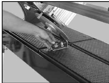
(E) Using a combination square, check the Blade for 45° alignment.
