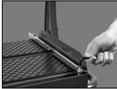
(B) Remove the Back Stop.
