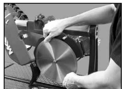
(I) Remove the old Diamond Blade.
