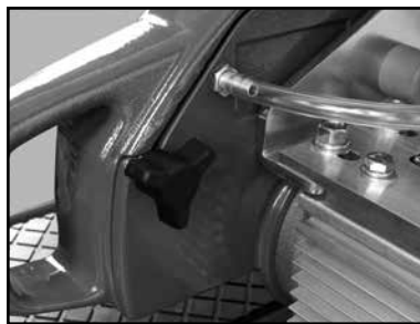
(E) Loosen the Blade Guard Retaining Knob.
