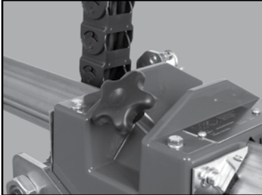
(A) Loosen the Cutting Head Locking Knob.
