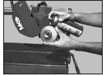
(C) Lubricate the Inner Flange Gasket.
