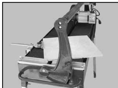
(E) Verify the tile is seated against the Stop and Protractor and that the desired angle is correct.
