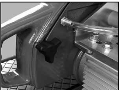
(G) Loosen the Blade Guard Retaining Knob.
