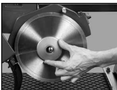
(H) Remove the Outer Flange.
