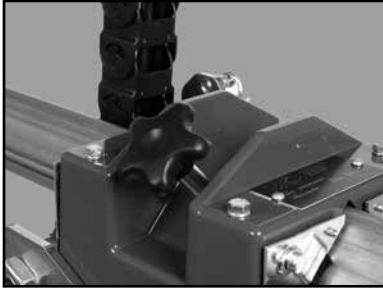
(A) Loosen the Cutting Head Locking Knob.
