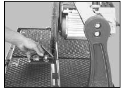
(C) Check the Cutting Head alignment.
