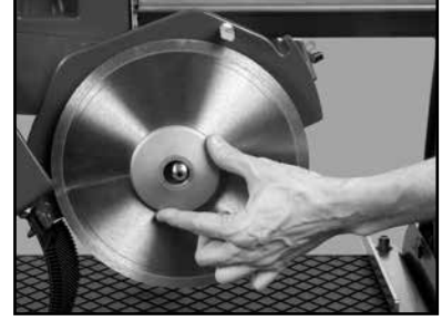
(L) Install the Outer Flange.
