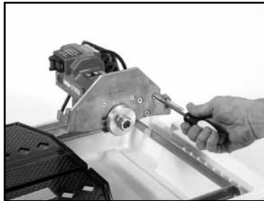
(E) Install the three Cutting Head Retaining Screws using a Phillips Screwdriver
