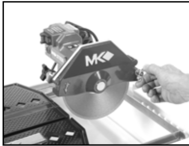
(H) Close the Blade Guard and tighten the Blade Guard Retaining Knob
