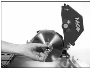
(G) Install the Outer Flange and Retaining Nut; install the Shaft Wrench and Blade Wrench as shown in Steps C and D and tighten the Retaining Nut
