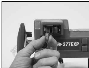
(B) Lockout the Saw by removing the Lockout Pin.
