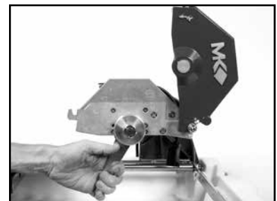
(C) Place the Shaft Wrench on the Motor Shaft rotate blade shaft so shaft wrench is engaged.
