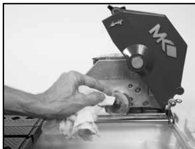
(B) Clean the Motor Shaft.
