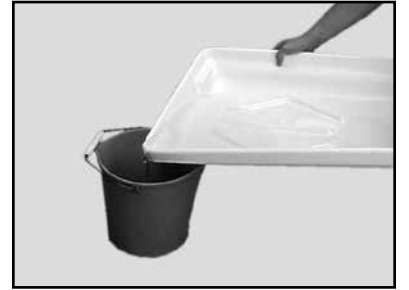
(F) Dispose of the contents of the Water Pan and clean the MK-377EXP with soap and clear water.
