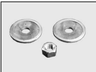
(A) Remove and clean the Inner and Outer Flanges and the Blade Retaining Nut.
