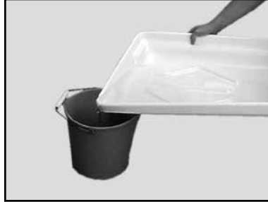
(B) Dispose of the contents of the Water Pan and clean the pan. Replace the Cutting Assembly.
