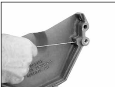
(G) Rod Cooling Channels and recheck flow.
