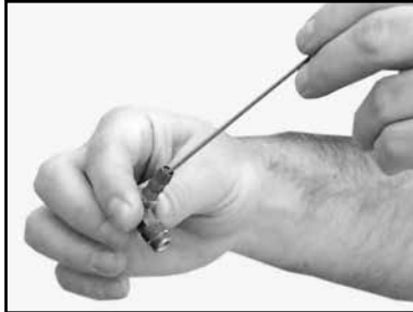
(E) Clean the Blade Guard Intake Fitting.
