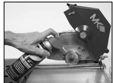
(C) Lubricate the Motor Shaft.
