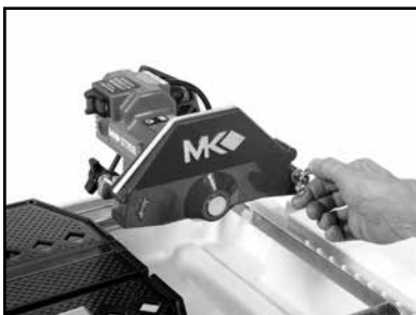
(A) Loosen the Blade Guard Retaining Wingnut.
