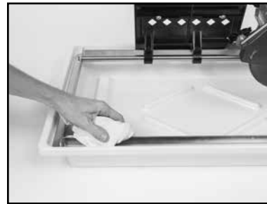
(H) Clean the Roller Wheel Guide Rail.
