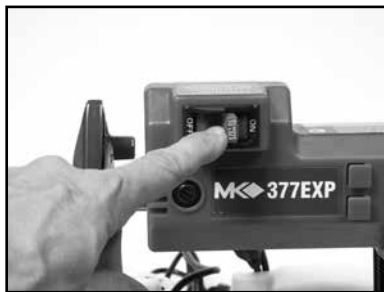
(A) Locate the Lockout Pin in the center of the ON/OFF Switch toggle (the Lockout Pin has "Remove To Lock" highlighted).
