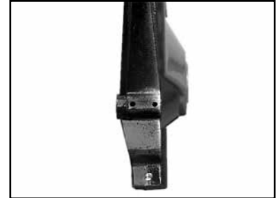
(F) Locate the Blade Guard Cooling Channels.
