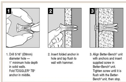
Direct fastening to studs or blocking is eliminated when using supplied hollow wall anchors, as shown .
