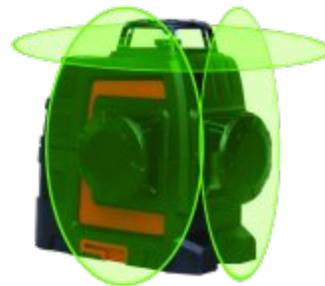
Johnson's ultra-bright green beam laser projects three self-leveling 360° planes of laser light for total jobsite coverage up to 200'. This laser offers 3 green beams – one horizontal and two vertical for one-person alignment, leveling and layout using one tool. Robust construction withstands tough jobsite conditions and provides resistance to dust and water. Pulse mode for use with separate detector in bright light or outdoor conditions where beams are not visible.
