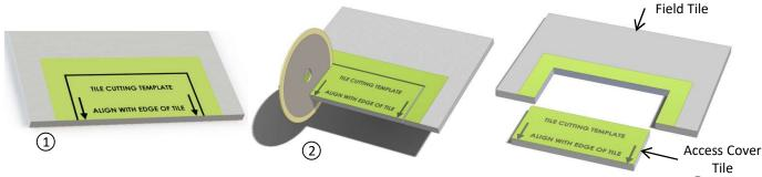
$\bigcirc$  Adhere the Cutting Template to the edge of the tile that aligns with the Access Opening.  $\bigcirc$  Cut precisely along the black line. (3) Remove the Access Cover Tile from the Field Tile. Cut precisely to the template. The Quick Dry Adhesive will not span large gaps. The Access Cover Frame should fit
