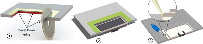
1 Lightly bevel the bottom edges of the Field Tile 1-5 degrees. 2 Install the Access Cover Tray and Frame into the cutout. (3) Turn over onto a flat surface, making sure the rim of the Access Cover Frame and Field Tile are flush. Apply Quick Dry Adhesive between the Field Tile and Access Cover Frame.
