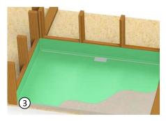
1.Install Debris Plugs 2.Caulk all joints and prepare for surface applied waterproofing membrane. 3.Apply waterproofing up walls/framing a minimum of 5". Follow all waterproofing manufacturer's recommendations.
