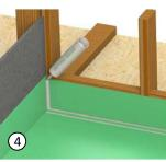
1.Coat all faces of wall tile backer up min of 5" with liquid waterproofing to prevent wicking. 2.Apply a generous bead of sealant at the floor/wall transition. 3. Embed the coated tile backer into the sealant and secure to the wall. 4. Apply sealant at the corner of the previously installed tile backer before installing the next piece.
