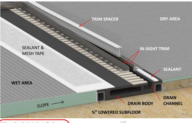
When the drain is installed at an entry, In-Sight Trims must be used. It is also highly recommended that a glass enclosure or small curb is placed at the entry to limit water escape.
