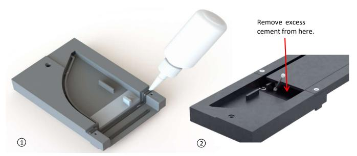
IMPORTANT: Apply two lines of ABS cement as shown to provide for air escape during assembly. If air is trapped by improper application, it can create a pathway for water escape.
