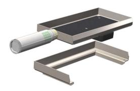
NOTICE: Use the supplied Wax Stick to wax the Access Cover Tray. Waxing the cover prevents accidental bonding of mortar or adhesive. It also prevents mineral build up and aids in future removal.
