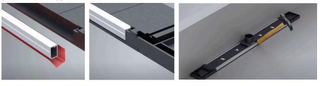
**Drill and Countersink for Rail Attachment Screws:** Use the Drill Guide, Countersink Guide, and Drill Bit to make six countersunk holes through the Drain Body and Rails. Screws should be roughly placed at each end and center of both Rails. Do not over-tighten the Screws.
