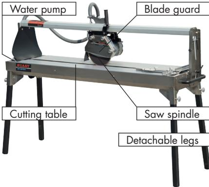
spindle. The saw flange is to be mounted on the saw spindle with a hexagon nut to clamp the saw blade.
