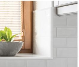
RONDEC-STEP edges out the tiled countertop while QUADEC frames out the tiled window ledge. DILEX-BWA replaces the need for grout between the countertop and wall tile.
