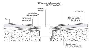
**Note**: This diagram is provided to show a typical drain detail and is not intended to make specific design recommendations.
