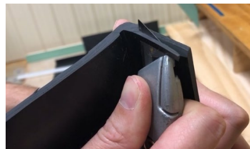
Figure 5: Undercut & bevel edge of finish cut
