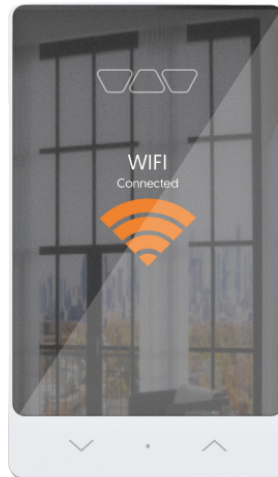
Wi-Fi connexion Press the up (^) and down (v) simultaneously and hold for 2 seconds to enter access point.
