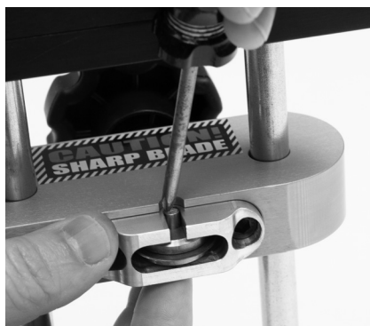
Step 6 - Center the Axle Pin using a screwdriver or pen.
