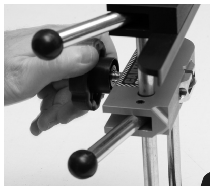
Step 7 - Turn the knob counterclockwise to return the blade to scoring position.
