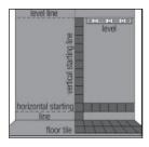
Determine whether floor is level by measuring distance to desired tile height on both sides of area to be tiled. If there is a difference (i.e., the floor is lower on one side), lay one vertical row of tile from desired tile height to low point of floor. Affix tiles with tilesetting materials. Use this first row as a guide to keep tiles and grout lines level and even throughout installation.
