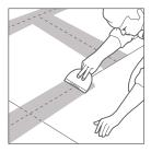
Fill joints with latex-fortified mortar or Type 1 organic adhesive and immediately embed USG Durock<sup>-</sup> tilebacker tape or equivalent alkaliresistant, fiberglass mesh joint tape.
