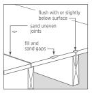
Clean subfloor and leave free of dust, dirt and debris, Ensure that subfloor is completely dry (no more than 12% moisture in subfloor prior to install). Verify that fasteners are flush with, or slightly below, subfloor surface.
