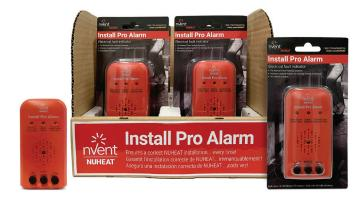
nVent NUHEAT Install Pro Alarm (AC0200) is an electrical fault indicator that simultaneously monitors the hot, neutral and ground wires during installation of any line voltage floor heating system. If a wire is damaged during installation, the Install Pro Alarm will sound an alert, prompting the installer to stop and correct the problem before continuing.
