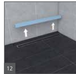
12 Remove the foam block spacer.
